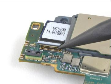
• Use the pointed end of a spudger to disconnect the ultra wide camera from the motherboard.
