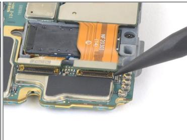
• Use the pointed end of a spudger to disconnect the wide-angle camera from the motherboard.
