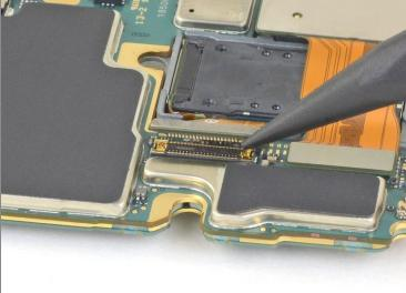
• Use the pointed end of a spudger to disconnect the telephoto camera from the motherboard.
