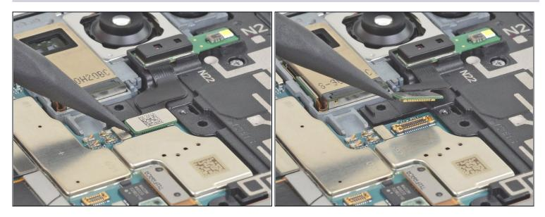
• Use the pointed end of a spudger to pry up the laser AF sensor press connector.
