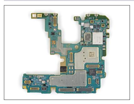
Only the motherboard remains. Compare your new replacement part to the original part—you may need to transfer remaining components or remove adhesive backings from the new part before installing.
