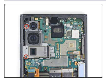
Use a Phillips screwdriver to remove the two 4.0 mm screws securing the motherboard to the frame.
