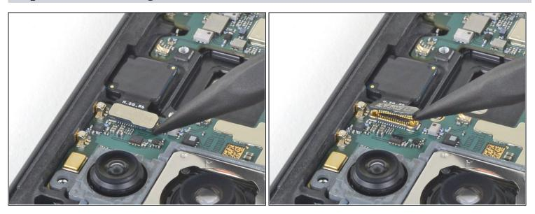
• Use the pointed end of a spudger to disconnect the front-facing camera cable from the motherboard.
