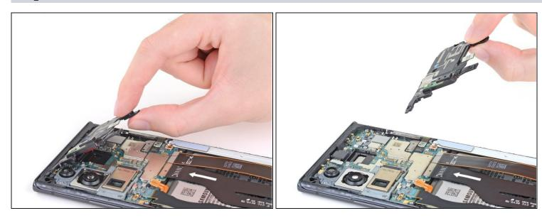
• Lift and remove the earpiece speaker.
