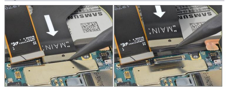
• Use the pointed end of a spudger to disconnect the main interconnect cable from the motherboard.
