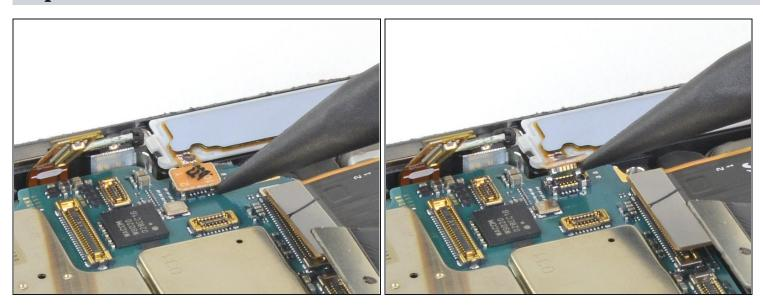
• Use the pointed end of a spudger to disconnect the S-Pen press connector from the motherboard.
