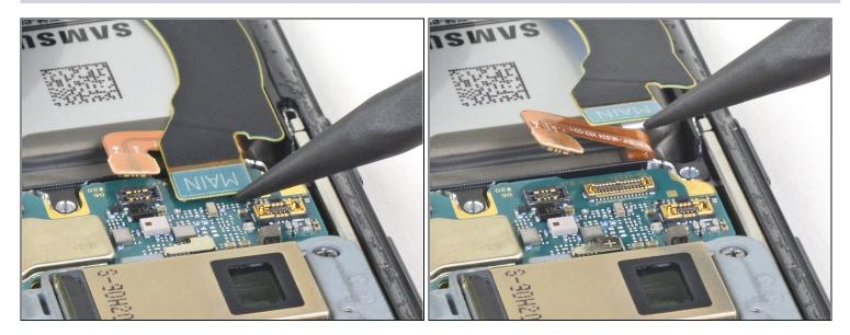
• Use the pointed end of a spudger to disconnect the secondary interconnect cable from the motherboard.
