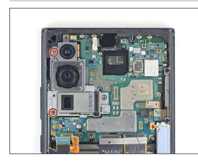
Use a Phillips screwdriver to remove the two 4.0 mm screws securing the motherboard to the frame.
