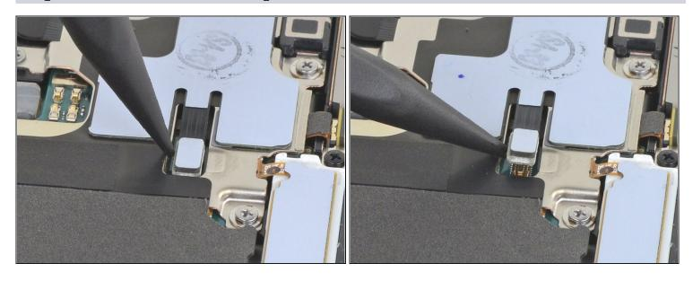
• Use the pointed end of a spudger to pry up and disconnect the white press connector located in the bottom right of the motherboard shield.
