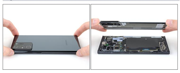
• Lift the rear cover straight up to remove it.
