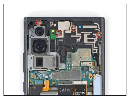
Use a Phillips screwdriver to remove the four 4.0 mm screws securing the earpiece speaker.
