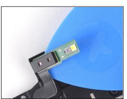
• Push the opening pick underneath the top of the laser AF sensor to cut through the adhesive.
