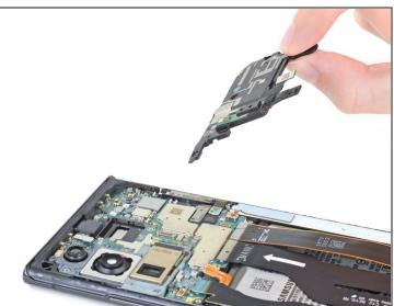
• Lift and remove the earpiece speaker.
