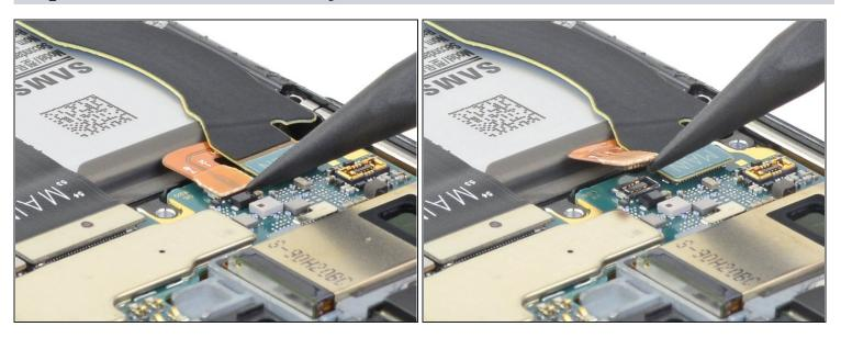
• Use the pointed end of a spudger to pry up the battery press connector to safely disconnect the battery before continuing repairs.
