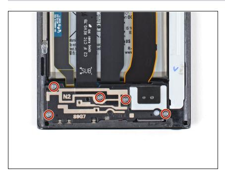
Use a Phillips screwdriver to remove the five 4.0 mm screws securing the loudspeaker to the frame.
