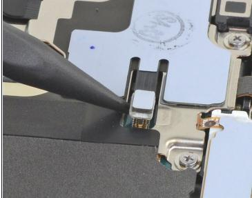
• Use the pointed end of a spudger to pry up and disconnect the white press connector located in the bottom right of the motherboard shield.
