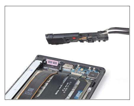
Use a pair of tweezers to lift and remove the loudspeaker. Compare your new replacement part to the original part—you may need to transfer remaining components or remove adhesive backings from the new part before installing.
