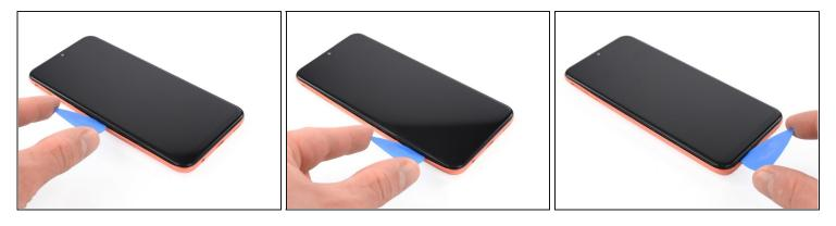
• Slide the opening pick around the bottom left corner to unclip the plastic clips.
