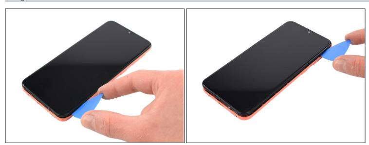
• Slide the opening pick along the right edge to the top right corner to unclip the plastic clips.
