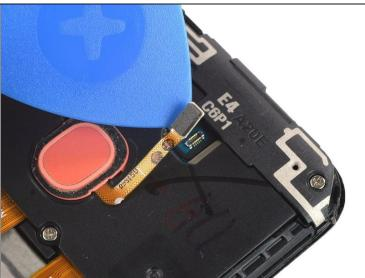
• Use an opening pick to pry up and disconnect the fingerprint sensor.
