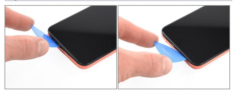
• Slide the opening pick along the bottom edge to unclip the plastic clips.
