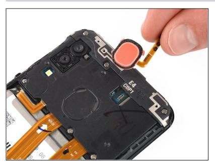
• Remove the fingerprint sensor.
