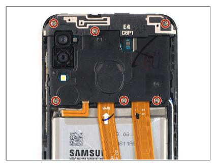
Use a Phillips screwdriver to remove the six 3.5 mm-long screws securing the motherboard covers.
