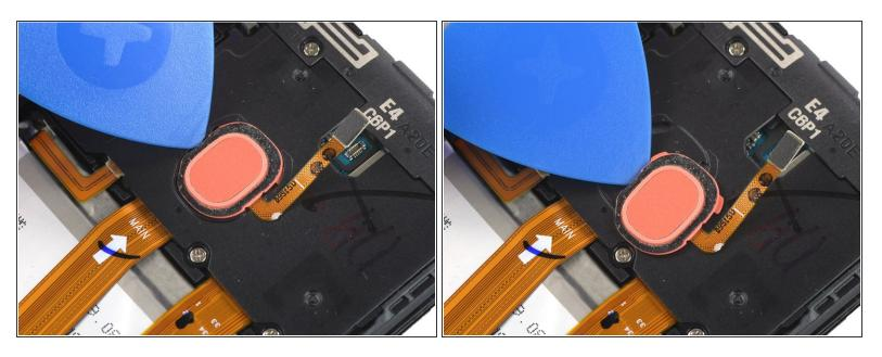
Push against the left edge of the fingerprint sensor with an opening pick to slide the sensor to the right and separate it from the motherboard cover.
