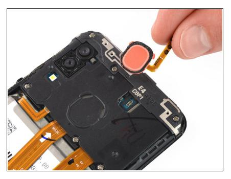
Remove the fingerprint sensor.
