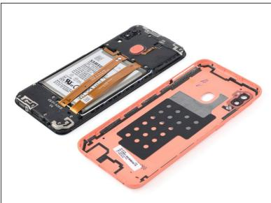
Separate the phone assembly from the back cover.
