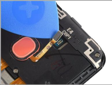
Use an opening pick to pry up and disconnect the fingerprint sensor.
