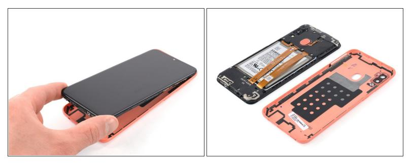
• Separate the phone assembly from the back cover.
