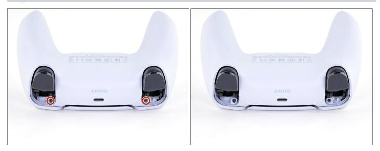
• Use a Phillips screwdriver to remove the two 6.4 mm screws behind the **L1** and **R1** buttons.
