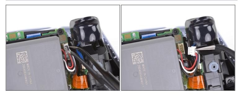
Use a pair of tweezers or your fingers to disconnect the battery from the motherboard.
