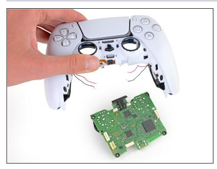
• Separate the controller from the motherboard.
