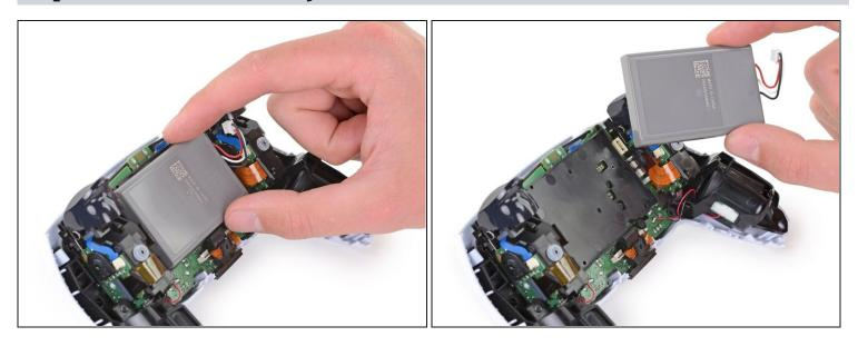
• Lift the battery straight out of the battery bracket.
