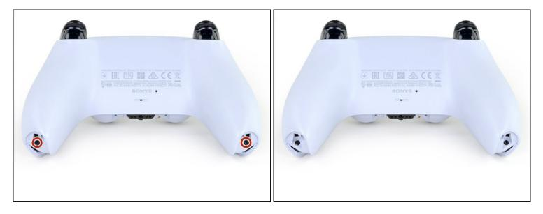
• Use a Phillips screwdriver to remove the two 6.4 mm screws securing the bottom corners of the lower case.
