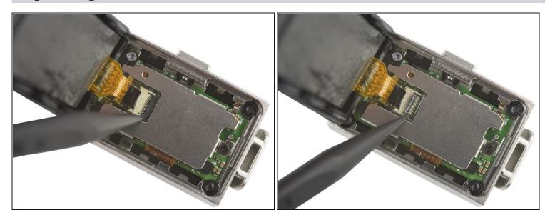
• Use the pointed end of a spudger to open the ZIF connector by pushing up the black flap.
