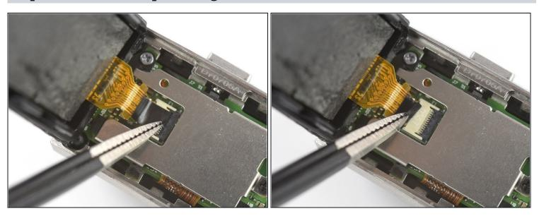
• Use a pair of blunt nosed <u>tweezers</u> to remove the black sticker which covering the touch screen connector.
