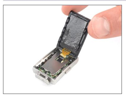
Carefully fold the touch screen assembly in the direction of the bottom edge.
