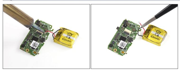
• Use a soldering iron to desolder the second battery cable from the motherboard.
