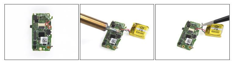
• Use a soldering iron to desolder the first battery cable from the motherboard.
