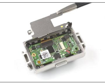
• Use a pair of blunt nose <u>tweezers</u> to remove the motherboard shield.
