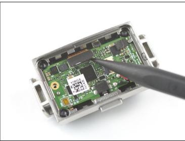
• Use the pointed end of a spudger to pry up and disconnect the heart rate monitor sensor flex cable.
