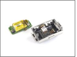
• Use an opening pick to pry up and remove the motherboard which is holding the battery.
