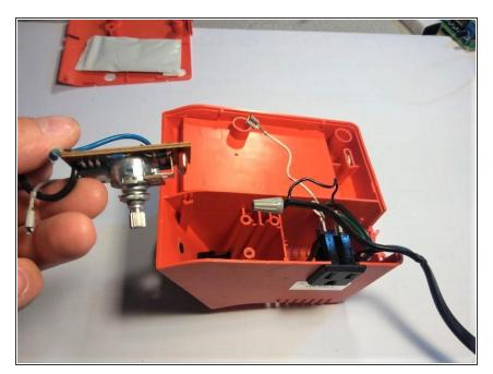
• Remove the adjustable heat dial board.
