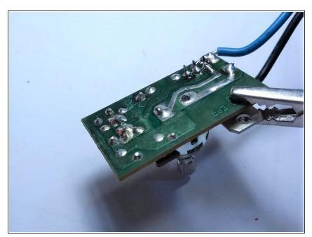
• Verify all three pins are soldered in and the solder is not touching the other pins.
