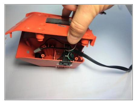
Replace the bottom and replace all four screws and rubber feet, reversing steps four though two.
