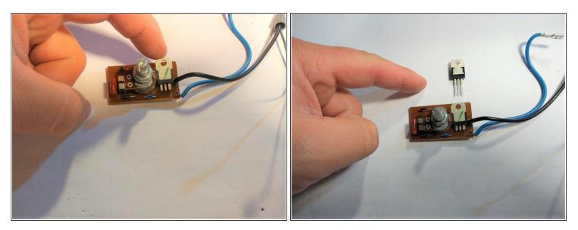
• Orient the new TRIAC switch the same way as the old TRIAC switch is located.
