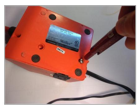
Remove two 8.6 mm Phillips #1 screws from soldering station bottom.
