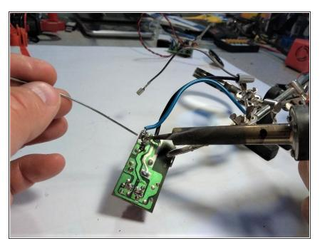
• Solder the new TRIAC switch onto board.
