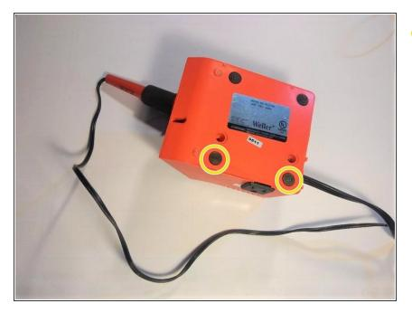
Remove the rubber feet to access the remaining screws.
