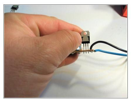
• Insert the new TRIAC switch into the three holes left when you removed the old TRIAC switch.
