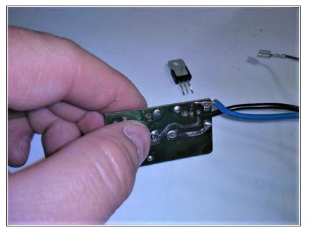
• Remove the TRIAC switch when all the solder is removed from the pins.
