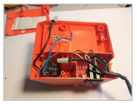
• Separate the bottom and top half of the soldering station.
