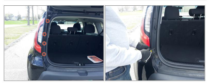
Use a Phillips #2 screwdriver to remove the four 20.0 mm screws from the tail light assembly.
