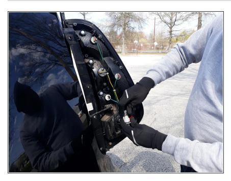
Press the light bulb down and turn it 1/4 counterclockwise.
