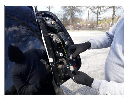
• Pull the light bulb out of the socket.
