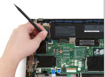
• Use the flat end of a spudger to flip the power button cable's black tab up.
