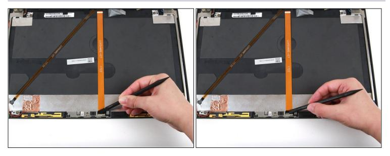
• Use the flat end of a spudger to flip up the black locking flap securing the ribbon cable.
