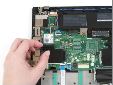
• Use a finger to press the black flap covering the Wi-Fi card down.
