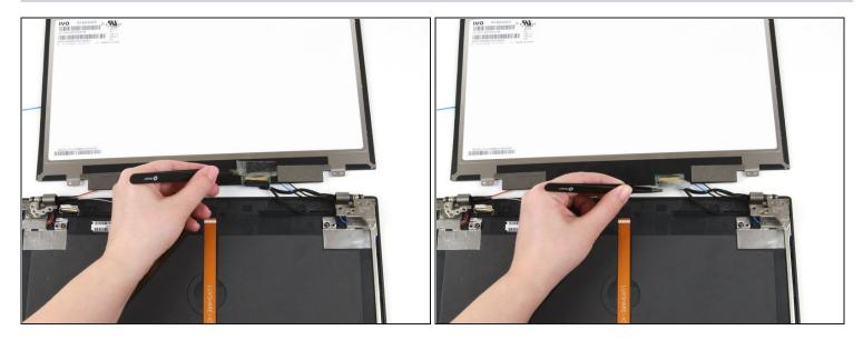
• Use a pair of blunt nose tweezers to remove the clear tape from the display cable.
