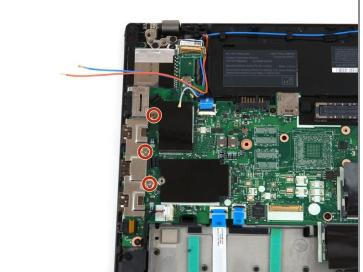
• Use a Phillips #1 screwdriver to remove the three 4 mm screws from the I/O bracket.
