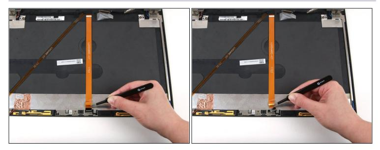
• Use a pair of blunt nose tweezers to slide the ribbon cable out of its connector.
