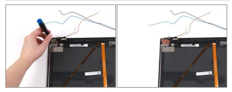
• Use a Phillips #1 screwdriver to remove the two 3 mm screws from the hinge in the upper left corner.
