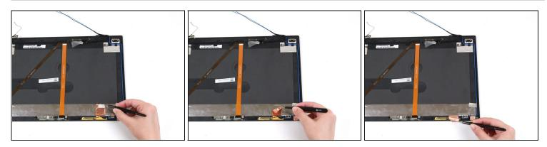
• Use a pair of blunt nose tweezers to peel the copper tape up from the display assembly in the bottom right-hand corner.
