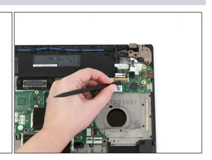
• Use the flat end of a spudger to flip up the metal bracket securing the camera cable to the motherboard.
