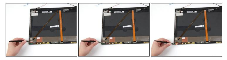
• Use a pair of blunt nose <u>tweezers</u> to peel the copper tape off of the hinge frame.
