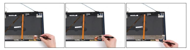
• Use a pair of blunt nose tweezers to peel the copper tape up from the display assembly in the bottom right-hand corner.
