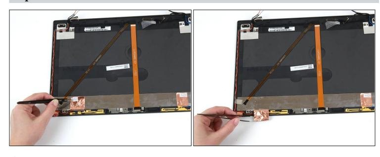
• Use a pair of blunt nose <u>tweezers</u> to peel the copper tape up from the display assembly in the bottom left-hand corner.
