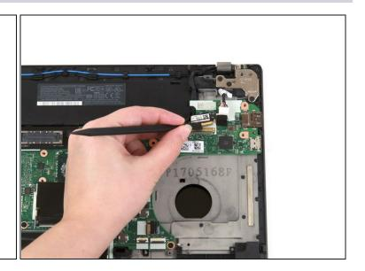
Use the flat end of a spudger to disconnect the camera cable from its socket on the motherboard.
