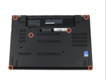
• Use a Phillips #1 screwdriver to loosen the six captive screws on the bottom cover of the laptop.
