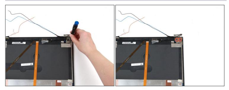
• Use a Phillips #1 screwdriver to remove the two 3 mm screws from the hinge in the upper right corner.
