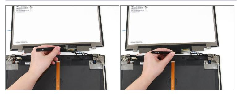
• Use a pair of blunt nose <u>tweezers</u> to remove the clear tape from the display cable.
