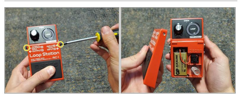
Using the Phillips #0 screwdriver, remove the two screws that secure the pedal to the device.
