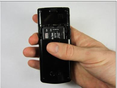
Use your thumb to press down and slide off the back cover of the phone.
