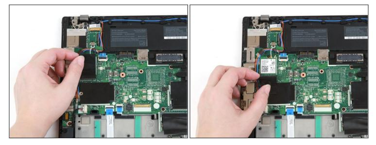
• Use a finger to press the black flap covering the Wi-Fi card down.
