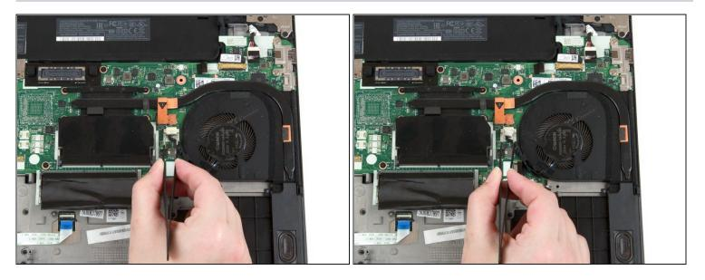
• Use a pair of blunt nose tweezers to pull the white fan connector out of its socket on the motherboard.
