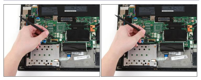
• Use the flat end of a spudger to flip up the metal clip securing the SSD connector to the motherboard.
