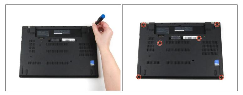
• Use a Phillips #1 screwdriver to loosen the six captive screws on the bottom cover of the laptop.
