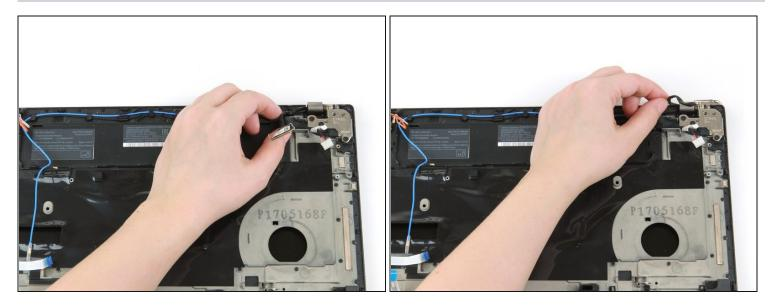
• Use your fingers to remove the camera cable from its slot.
