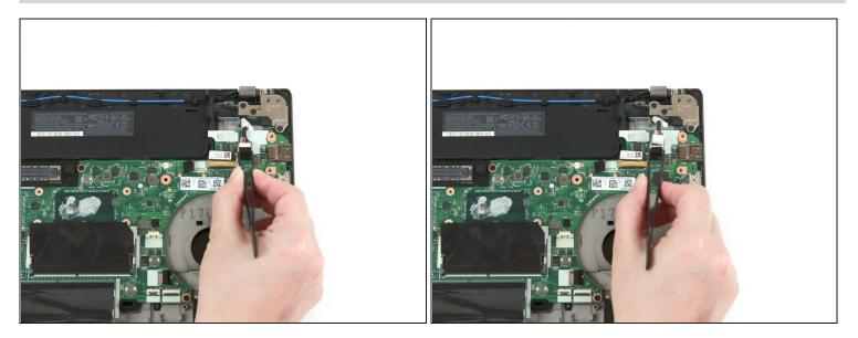
• Use a pair of blunt nose <u>tweezers</u> to disconnect the DC-in cable from its socket on the motherboard.
