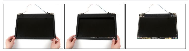
• Use both hands to lift the bezel up and away from the display assembly.
