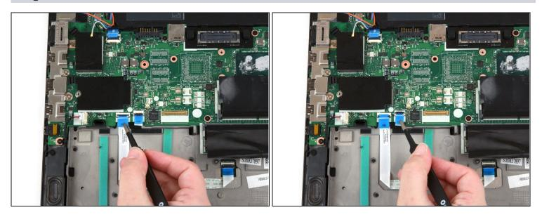
• Use a pair of blunt nose tweezers to slide the trackpad and fingerprint reader cables out of their connectors on the motherboard.
