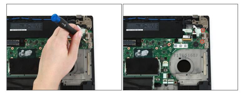
• Use a Phillips #1 screwdriver to remove the two 4 mm screws from the USB bracket.
