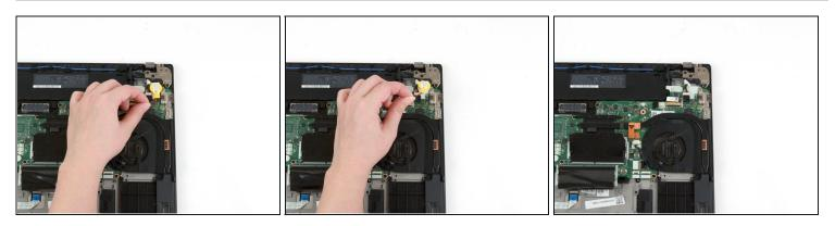
• Grab the wire attached to the coin cell battery, and lift it up and out of the laptop.
