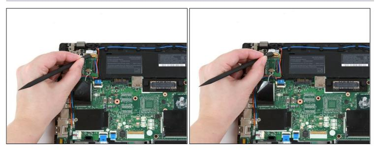
• Use the flat end of a spudger to disconnect the LCD cable from its socket on the motherboard.
