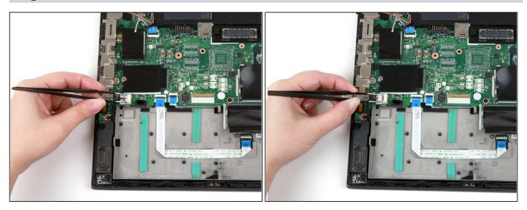
• Use a pair of blunt nose tweezers to disconnect the speaker cable from its socket on the motherboard.
