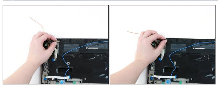
• Use your fingers to lift the LCD cable out of its slot.
