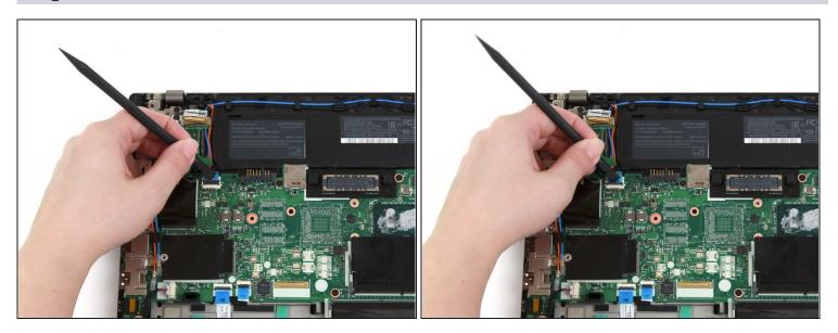
• Use the flat end of a spudger to flip the power button cable's black tab up.
