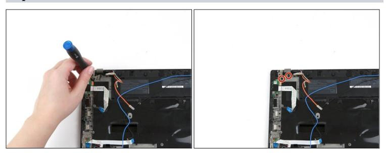
• Use a Phillips #1 screwdriver to remove two 4.5 mm screws from the hinge in the upper left corner.
