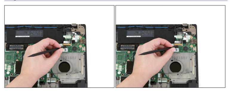
• Use the flat end of a spudger to flip up the metal bracket securing the camera cable to the motherboard.
