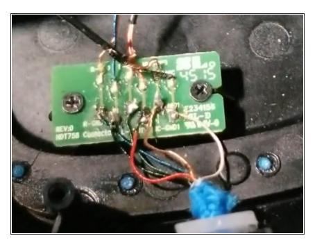
After you have finished soldering all connections, test the headset by plugging it into a computer, and check each speaker and the mic. If it still doesn't work, you may not have soldered it correctly, or there might be another problem in the headset or cable.
