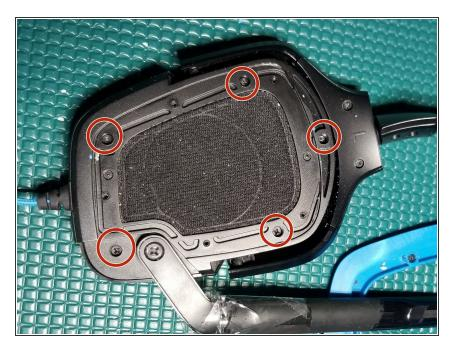
Insert and tighten the bottom layer of screws using a Phillips #1 screwdriver.
