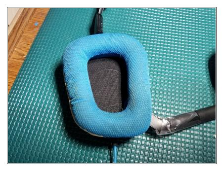
Pull the top-left corner of the foam padding up and to the left, and then pull it away from the frame.
