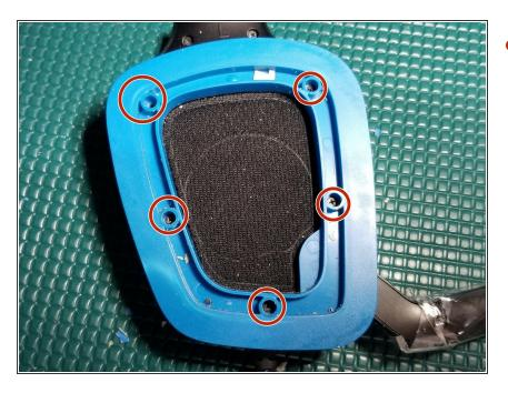
Insert and tighten top layer of screws using a #1 Phillips screwdriver.
