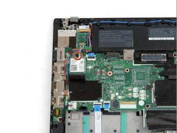
• Use a Phillips #1 screwdriver to remove the single 4 mm screw from the Wi-Fi card.
