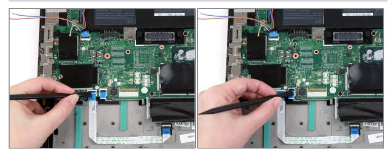
• Use the flat end of a spudger to flip up the black tabs on the trackpad and fingerprint reader cables.
