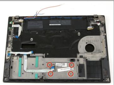
Use a Phillips #1 screwdriver to remove the four 4 mm screws.
