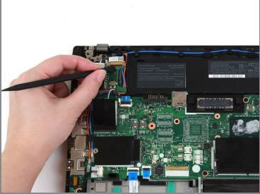
• Use the flat end of a spudger to flip up the metal clip securing the LCD cable to the motherboard.
