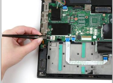
• Use a pair of blunt nose tweezers to disconnect the speaker cable from its socket on the motherboard.
