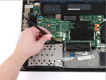
• Use the flat end of a spudger to separate the connector from its socket.
