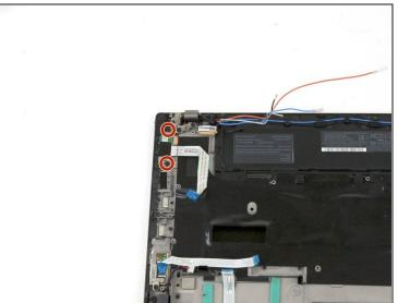
• Use a Phillips #1 screwdriver to remove the two 4 mm screws from the power button board.
