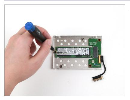
• Remove the single 4 mm screw using a Phillips #1 screwdriver.
