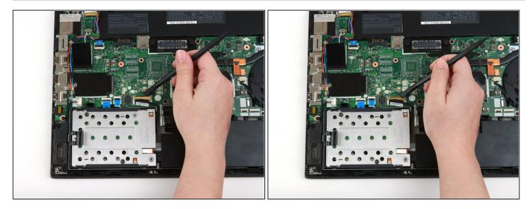
• Use the flat end of a spudger to flip up the metal clip securing the SSD connector to the motherboard.
