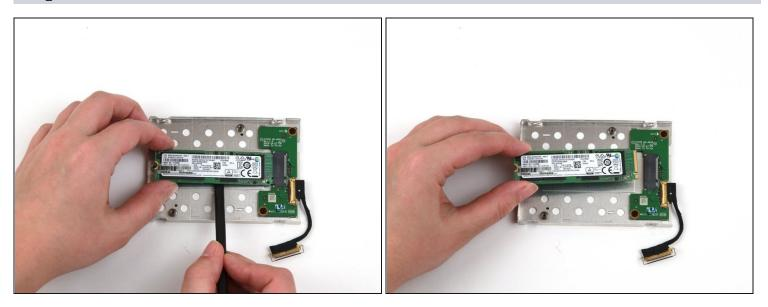
• Use the flat end of a spudger to pry the SSD up slightly and pull it out of the slot with your other hand.
