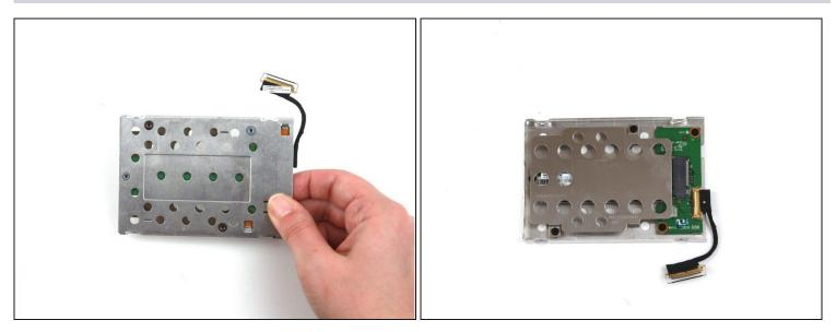
• Flip the SSD assembly over so that the green connector board is visible.
