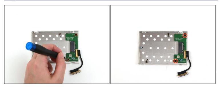
• Remove the two 4 mm screws from the SSD connector board using a Phillips #1 screwdriver.
