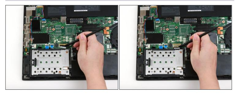
• Use the flat end of a spudger to separate the connector from its socket.
