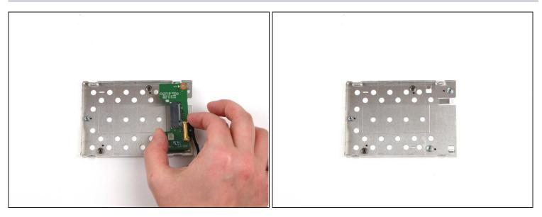
• Use your hand to remove the SSD connector board from the metal enclosure.
