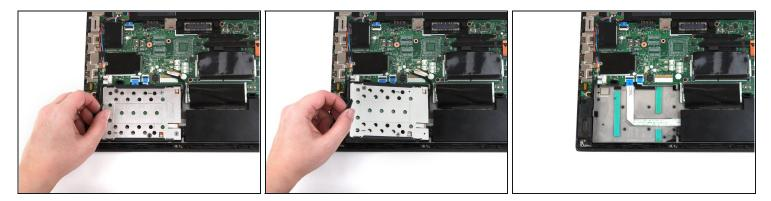
• Grab the tab on the left side of the SSD assembly, and pull up to remove it from the laptop.
