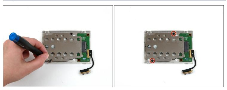
• Use a Phillips #1 screwdriver to remove the two 4 mm screws from the metal bracket.
