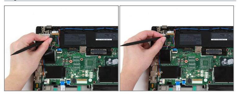
• Use the flat end of a spudger to flip up the metal clip securing the LCD cable to the motherboard.
