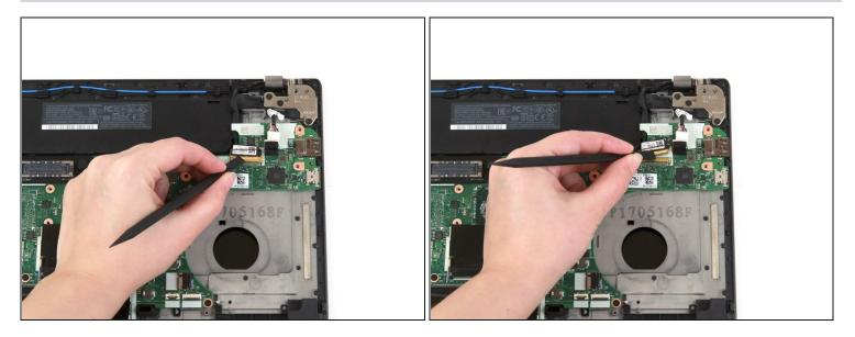
• Use the flat end of a spudger to disconnect the camera cable from its socket on the motherboard.
