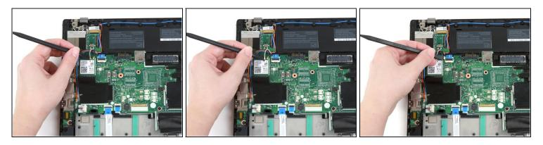
• Use the flat end of a spudger to disconnect the two coaxial wires from the Wi-Fi card.
