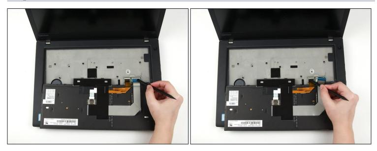
• Use the flat end of a spudger to flip up the locking flaps securing each of the two ribbon cables.
