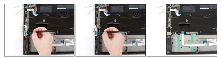
• Use the flat end of a spudger to pry the fingerprint reader up and away from the laptop.
