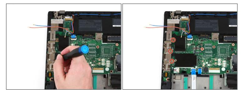
• Use a Phillips #1 screwdriver to remove the three 4 mm screws from the I/O bracket.
