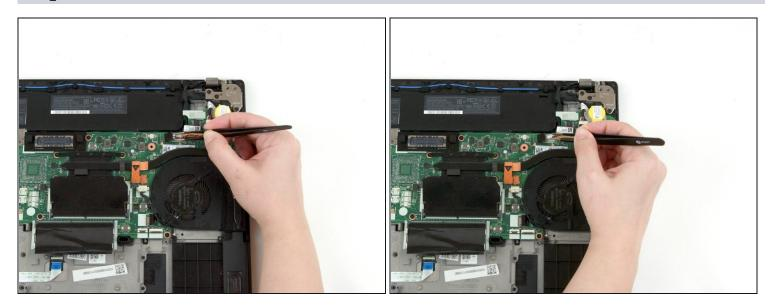
• Use a pair of blunt nose tweezers to pull the white connector out of its socket.
