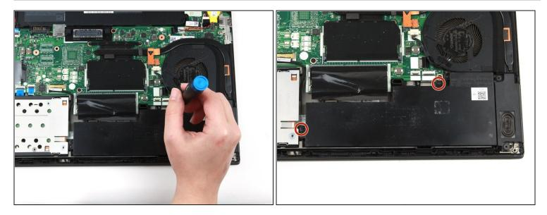
• Use a Phillips #1 screwdriver to remove two 5 mm screws from the internal battery.
