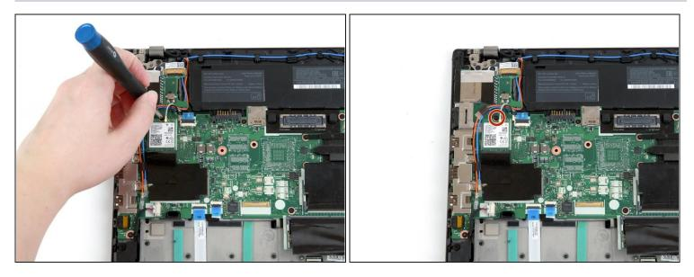
• Use a Phillips #1 screwdriver to remove the single 4 mm screw from the Wi-Fi card.
