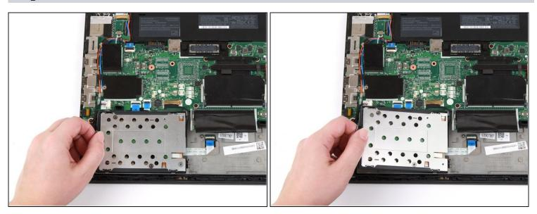
• Grab the tab on the left side of the hard drive, and pull up to remove it from the laptop.
