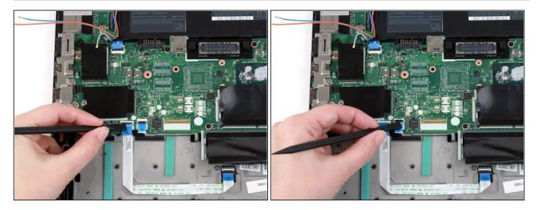
• Use the flat end of a spudger to flip up the black tabs on the trackpad and fingerprint reader cables.
