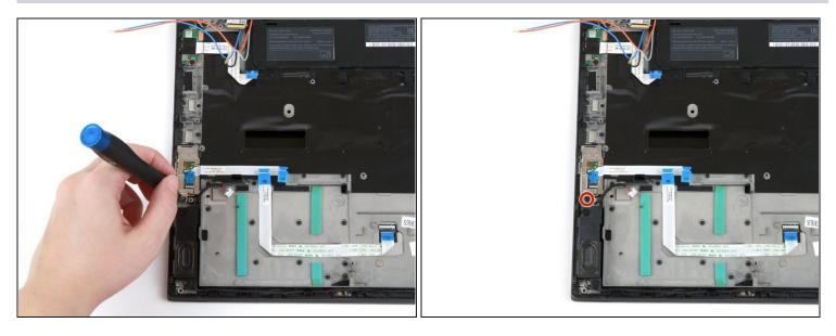
• Use a Phillips #1 screwdriver to remove the single 4 mm screw from the fingerprint reader bracket.
