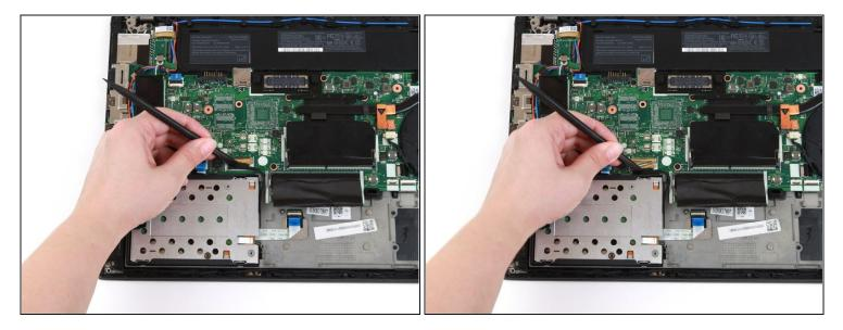
• Use the flat end of a spudger to separate the connector from its socket.
