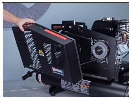
Tilt the belt guard away from the device and lift it out to remove it.
