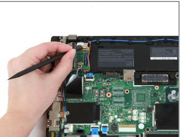
• Use the flat end of a spudger to disconnect the LCD cable from its socket on the motherboard.
