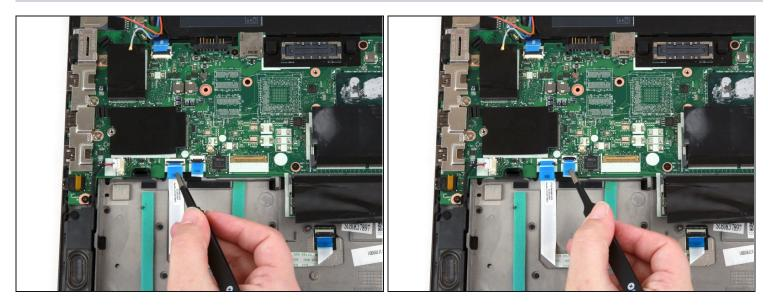
• Use a pair of blunt nose tweezers to slide the trackpad and fingerprint reader cables out of their connectors on the motherboard.
