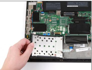
• Grab the tab on the left side of the hard drive, and pull up to remove it from the laptop.
