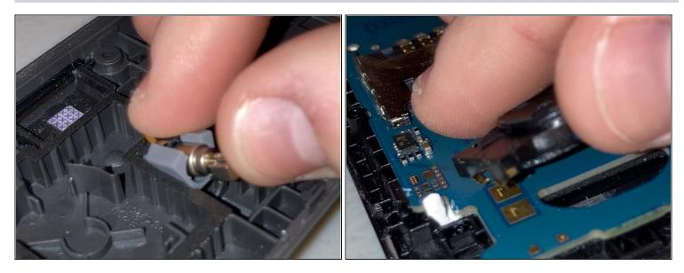
• On the back of the phone, we can remove the vibration motor and then on the circuit board, you can remove the speaker.
