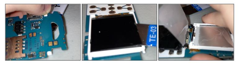
• Now, unclip the two white clips on the board, flip the board over and ever so carefully push an opening tool UNDER the screen and lift, CAREFULLY! Then remove the white plastic piece that WAS under the screen.
