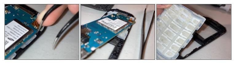
• Now, pull up on the top of the board, use <u>tweezers</u> to push the bottom right clip in, and then pull the board to the right and up. Next, remove the fake keypad.
