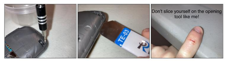
• Now, unscrew the three Phillips screws with a PH#000 screwdriver and use an opening tool to work your way around the edges to get the back-off.
