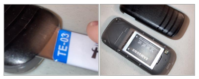
• For a more effortless experience, use an opening tool to remove the back. Simply push the opening tool into the indent in the bottom and work your way around a little so you can pop it off.
