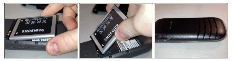
• Remove the battery by pulling it out, replacing it with a new one, and putting the cover back on.
