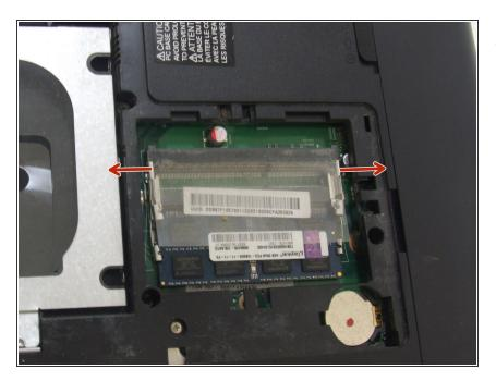
Spread the metal clamps on either side of the RAM card outward so the RAM pops up.
