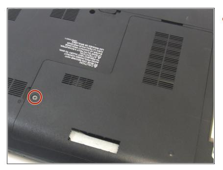
Unscrew the Phillips #00 screw, and remove the back cover.
