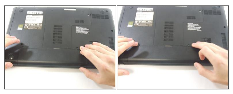
• Slide the two lock tabs on the battery to the open position.
