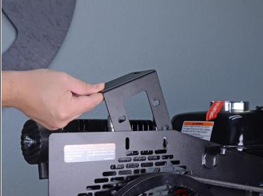
Lift the belt guard bracket straight up to remove it.
