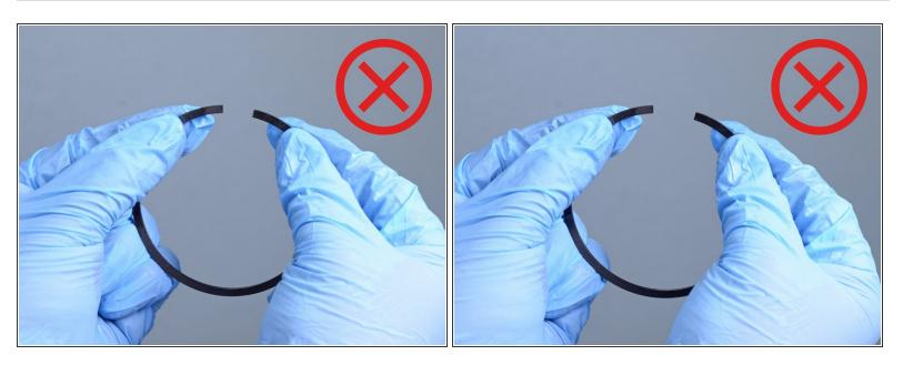
The composite compression and wiper rings are not designed to be bent in a way that moves their ends horizontally away from one another. Doing so excessively may cause the rings to break.
