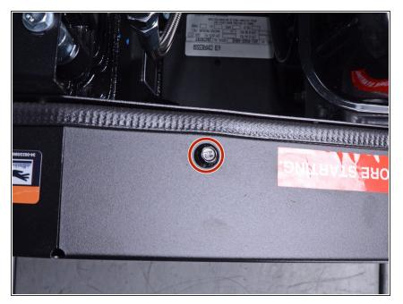
Use a 10 mm socket to remove the bolt securing the belt guard.
