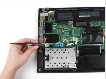
• Use a pair of blunt nose <u>tweezers</u> to remove the speaker connector from its socket.
