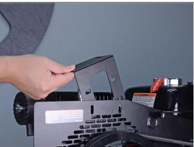
Lift the belt guard bracket straight up to remove it.
