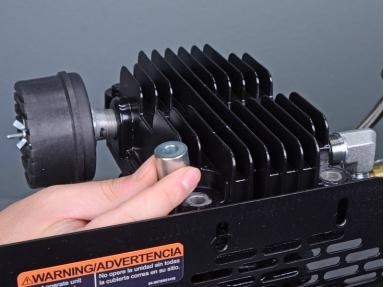
Remove the four spacers from the top of the cylinder head.
