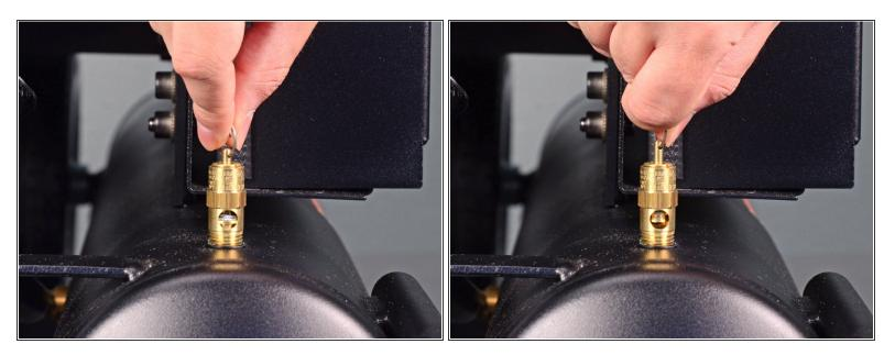
Pull the ring on the safety relief valve away from the compressor tank to drain the air from the compressor.
