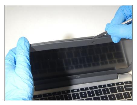
Insert your spudger between the plastic covering and the back of the case.
