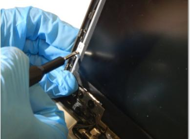
• Using a Phillips #0 Screwdriver, remove the four 2.5mm screws holding the screen in place.
