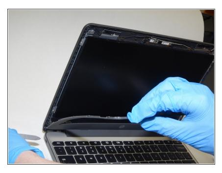
With the help of your spudger completely remove the plastic cover from the rest of the case.
