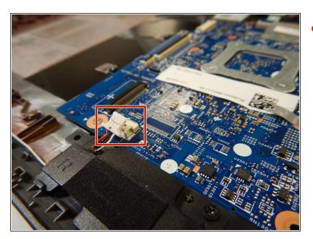
Remove the wire connecting the right speaker and motherboard.
