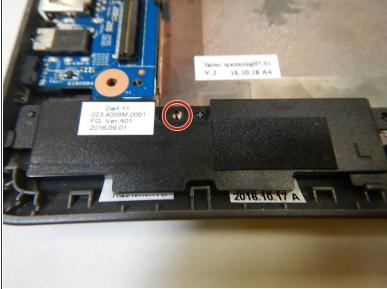
Using a Phillips #0 Screwdriver, remove the single 5mm screw connecting the left and right speakers to the casing.
