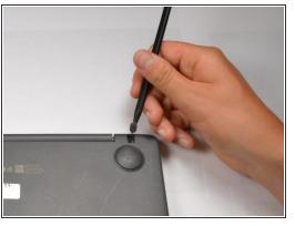
Using a sharp tool, remove the six adhesives from the bottom of your laptop to expose the screwheads underneath. Two of the pads are small and four are larger.
