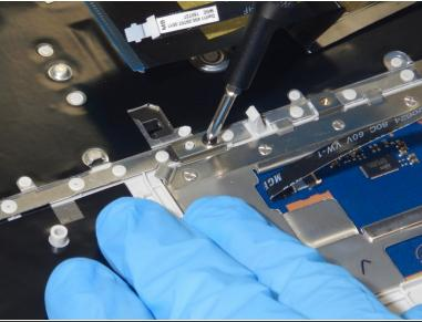
Using the Phillips # 0 Screwdriver, remove the three 2.5mm screws on the top of the trackpad.
