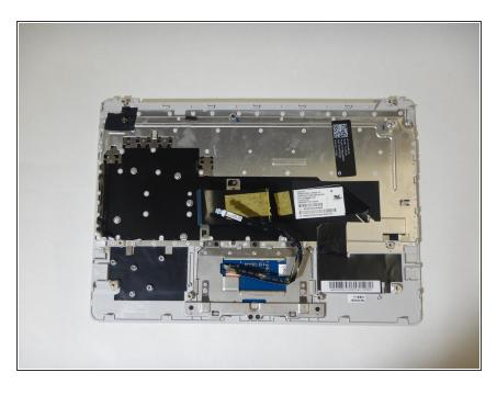
Remove the keyboard and reveal the underside.
