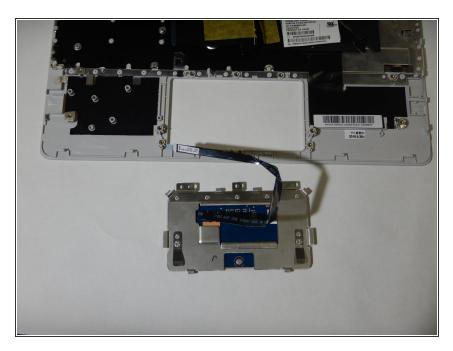
Gently lift the trackpad out of the casing.
