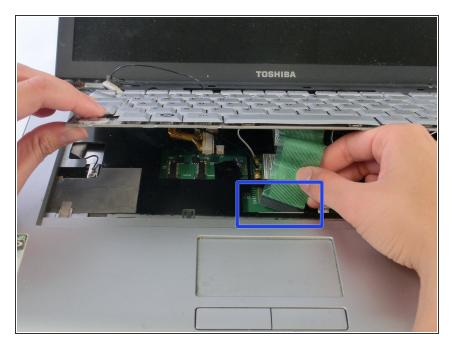
Disconnect the keyboard ribbon cable and remove the keyboard from the laptop.
