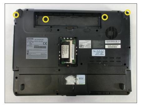
Unscrew the 4 highlighted screws with a PH1 screwdriver.
