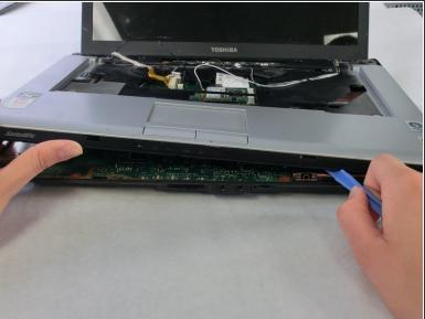
Slide the plastic opening tool underneath the edges of the upper casing, which is shown in the images.
