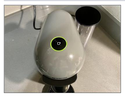
A green light will show, indicating the descaling has been completed successfully.
