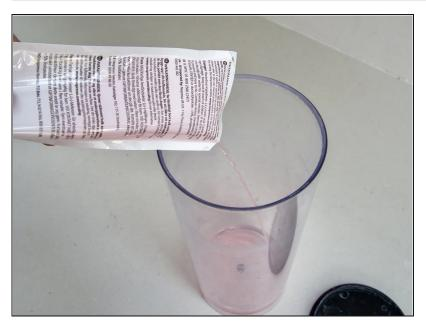
Fill the water tank with one unit of the Nespresso descaling liquid and add three cups of water to the solution.
