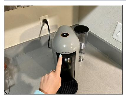
• To access the descaling mode, press the lever down one time.
