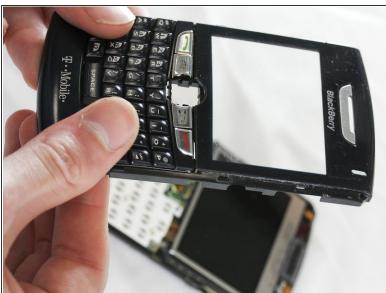
Slide the new keyboard into the casing. If done correctly, it should click into place and stay secure.
