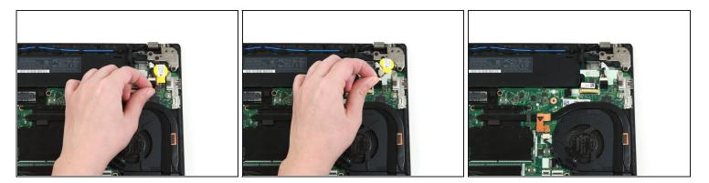
• Grab the wire attached to the coin cell battery, and lift it up and out of the laptop.
