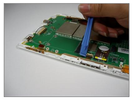
• Locate the next brown connector three inches to the right of the previous connector and repeat Step 10 to remove the plastic ribbon.
