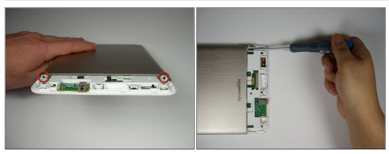
• Use a Phillips #00 screwdriver to remove the two 4 mm screws from the metal casing.
