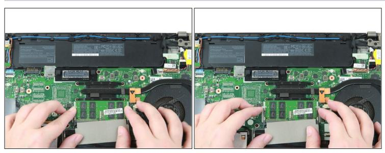
• Use your fingers to push the metal clips on either end of the RAM outwards.
