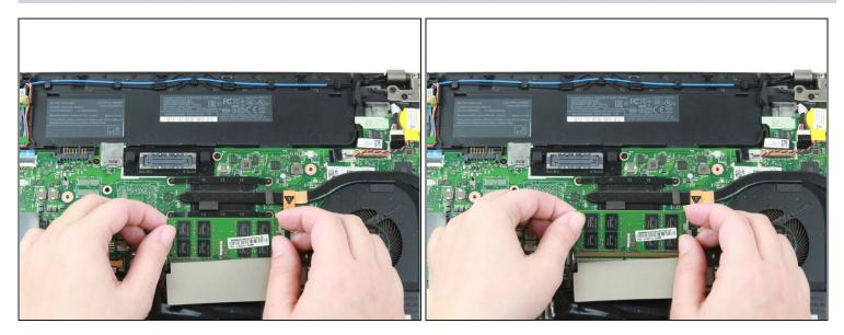
• Use your fingers to lift the RAM out of its socket and away from the laptop to remove it.
