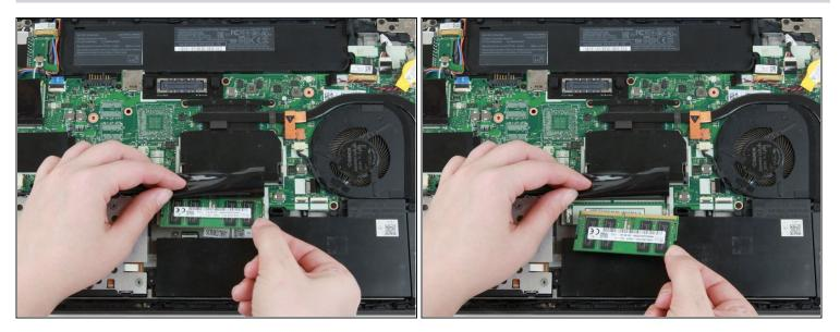
• Use your fingers to lift the RAM out of its socket and away from the laptop to remove it.
