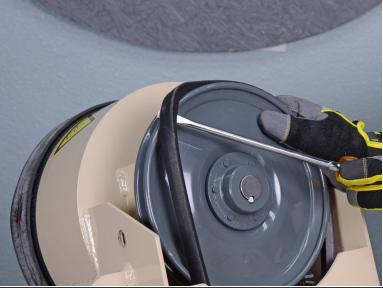
Continue to rotate the sheave with once hand while holding the flathead screwdriver with the other to fully dislodge the belt from the groove.
