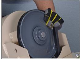
Reassembly tip: place the belt over the rim and rotate the sheave to guide the belt into the groove.
