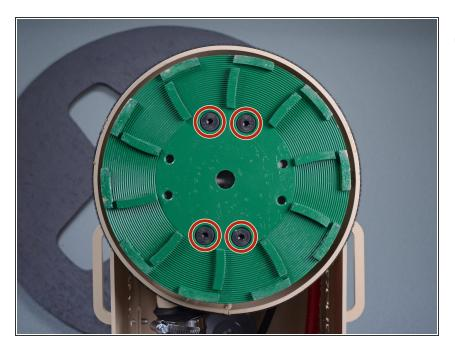
Use a 7/32 inch hex key to remove the four flat screws securing the disk to the head assembly.
