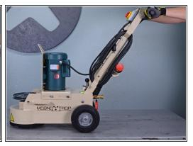
Tilt the machine back into working position.
