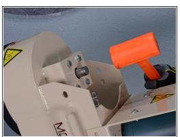
Use a dead blow hammer to hit the head assembly shaft straight down until it is flush with the upper bearing bracket, or as far as it will go.
