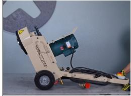
Tilt the front of the machine up off the ground.
