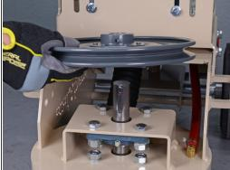
Lift the sheave straight up off of the head assembly shaft.
