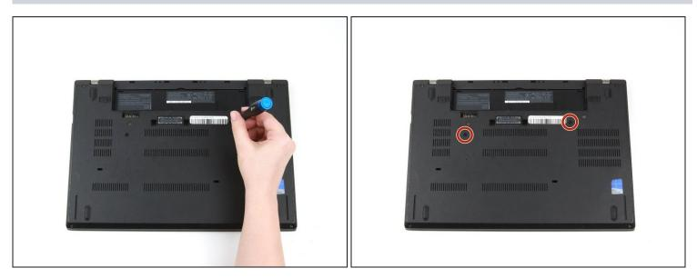
• Loosen the two captive Phillips #1 screws on the back cover of the laptop.
