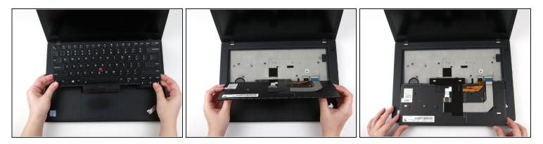
• Grab the bottom edge of the keyboard with your hands, and flip the keyboard upside-down, so it rests on the bottom of the laptop.
