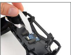
• Push the light diffuser through the inside of the rear case and remove it.
