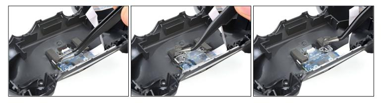
• Peel both foam pads from the light guide.
