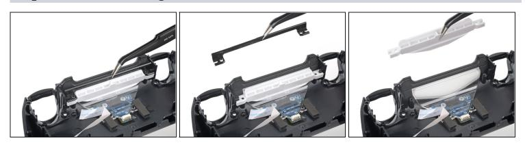
• Remove the black spacer and white bracket from the light guide.
