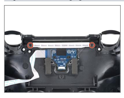
Use your Phillips screwdriver to remove the two 6.4 mm screws securing the light guide bracket to the rear case.
