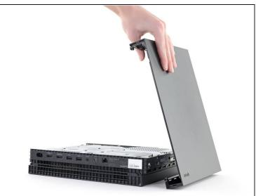
Push the upper plastic case down and away from the console to remove it completely.
