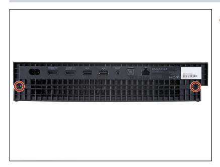
Use a T10 Torx screwdriver to remove the two 12.6 mm—long screws located on the back of the console.
