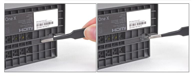
Use blunt tweezers to peel off the sticker covering the right-side screw on the back of the console.
