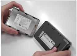
Push the black button and slide the battery casing to the left simultaneously, until the battery is completely separated from the device.
