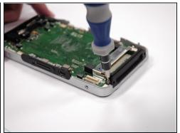
• Remove 2 screws (3.5 mm) on the black compact flash input using a Phillips #0.
