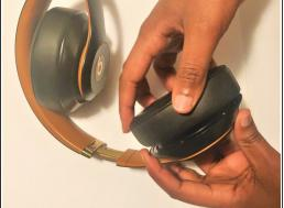
Realign and move as needed to match the circles on the adhesive on the earpad with the screws on your headphones.
