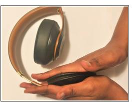
Once aligned and placed properly, push on your pad for 1 minute to activate the adhesive by clamping your hands together as tight as possible.
