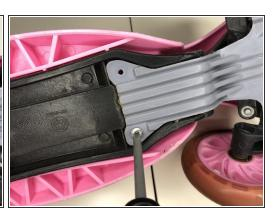
Remove the two bottom 16 mm pan head screws using a Phillips #1 screwdriver.
