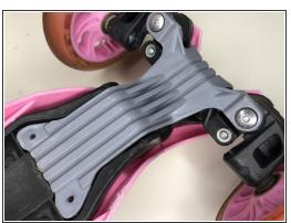
Insert and tighten the two 12 mm button head screws on top using a 4 mm Allen wrench.
