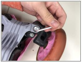
Remove the two 12 mm button head screws on top using a 4 mm Allen wrench.
