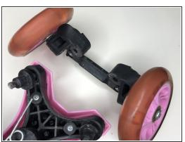
Carefully pull the sides of the wheels up and remove them from the spring.
