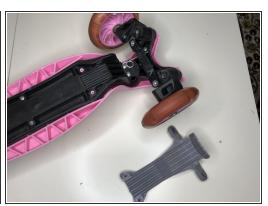
Remove the plastic case from the base of the scooter.
