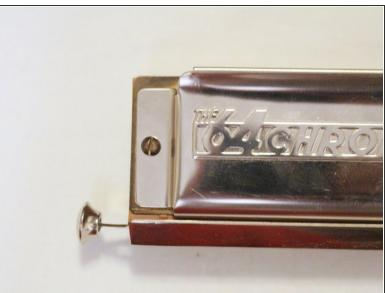
Slot one of the hollow round head screws into the aligned holes.
