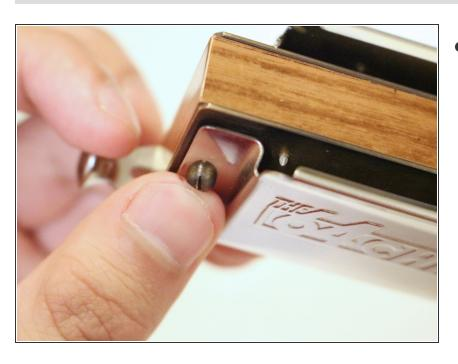
Keep the hollow round head screw in place by pressing down on the screw with your finger, resting the harmonica on a table, etc.
