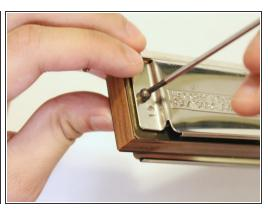
Using the screwdriver, screw one of the round head screws into the opposite hollow round head screw. Leave enough slack that the plate does not rise.
