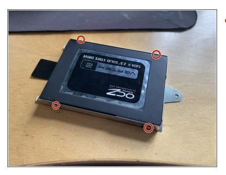
Remove 4 phillips screws to remove drive from caddy
