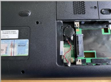
Disconnect CMOS battery backup connector from bottom of laptop
