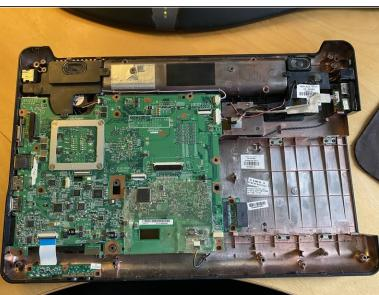
Lift top base off of laptop, being careful to disconnect the touchpad ribbon cable
