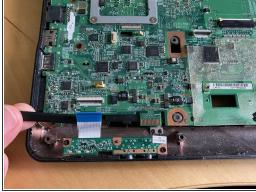
Lift audio/status light connector tab using a spudger and remove ribbon cable
