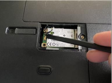
Using a spudger, remove the lower aerial cable
